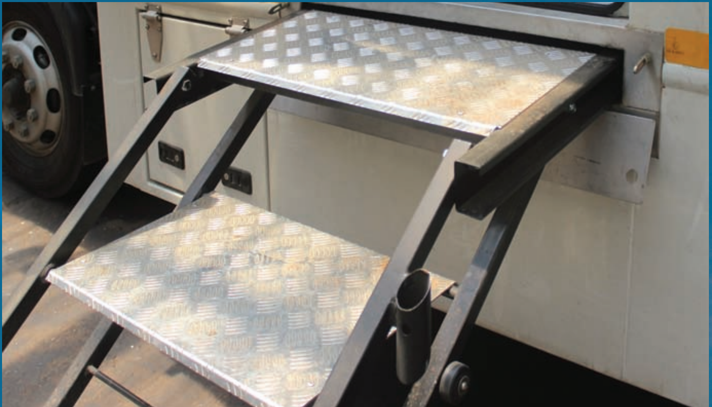
The vans feature sliding stowaway steps with skid-proof surfaces
