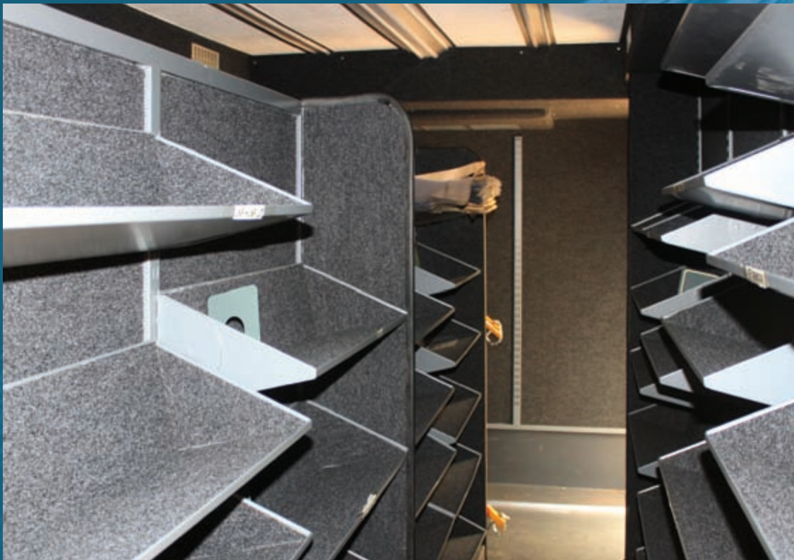
Shelves are adjustable and removable and lined with carpet to protect and secure books during transit
