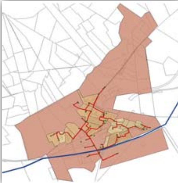
FIGURE 51: DE DOORNS SUPPLY AREA AND DISTRIBUTION NETWORK
