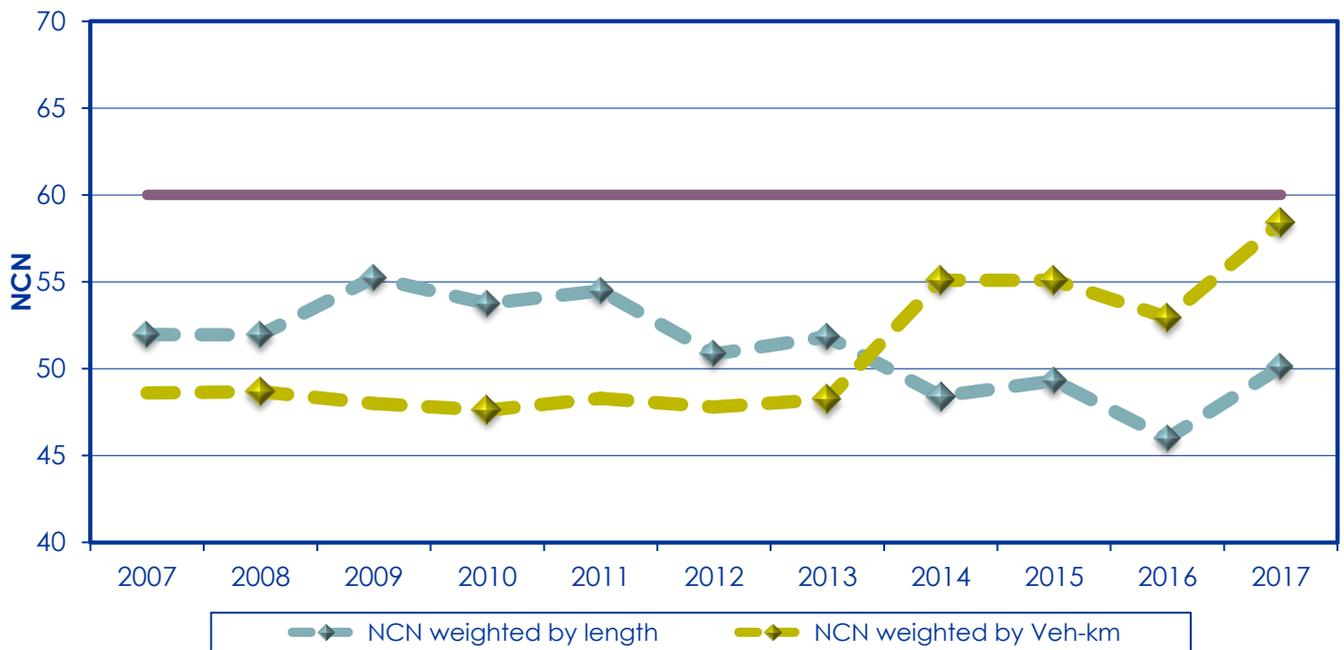
**Figure 4-27: The historic trend in the overall network condition of maintained unpaved roads 2007 to 2017**
