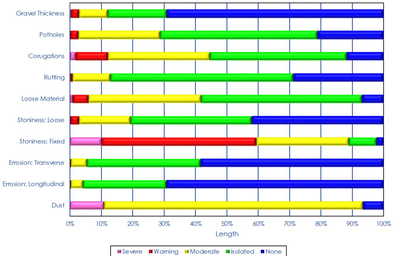
Figure 4-17: Condition distribution of the distresses on the unpaved road network as at June 2017
