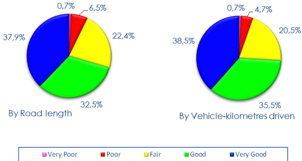
**Figure 4-2 Distribution of the VCI of paved roads by road length and vehicle-km as at June 2017**
