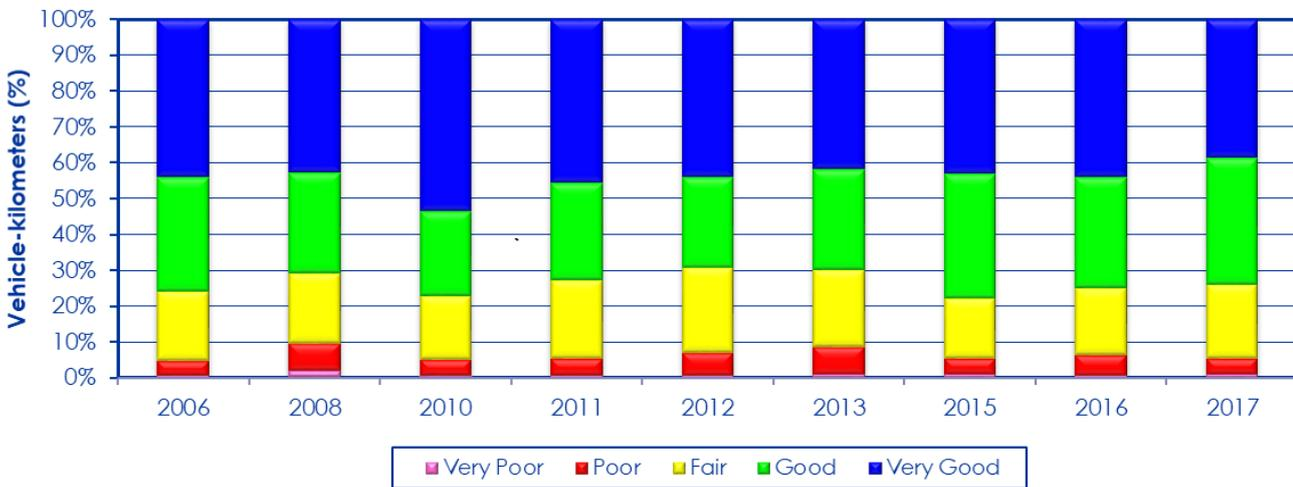
Figure 4-22: Distribution of the VCI of paved roads by annual vehicle-km travelled 2006-2017
