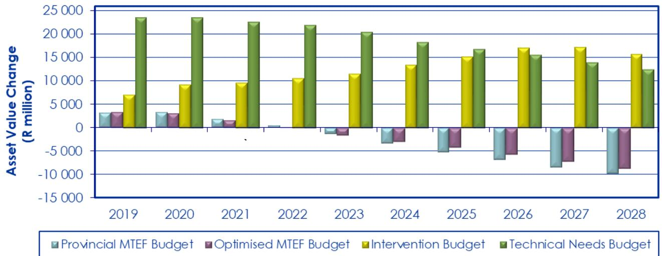
**Figure 5-40: Change in asset value of the road network compared to 2018 values**
