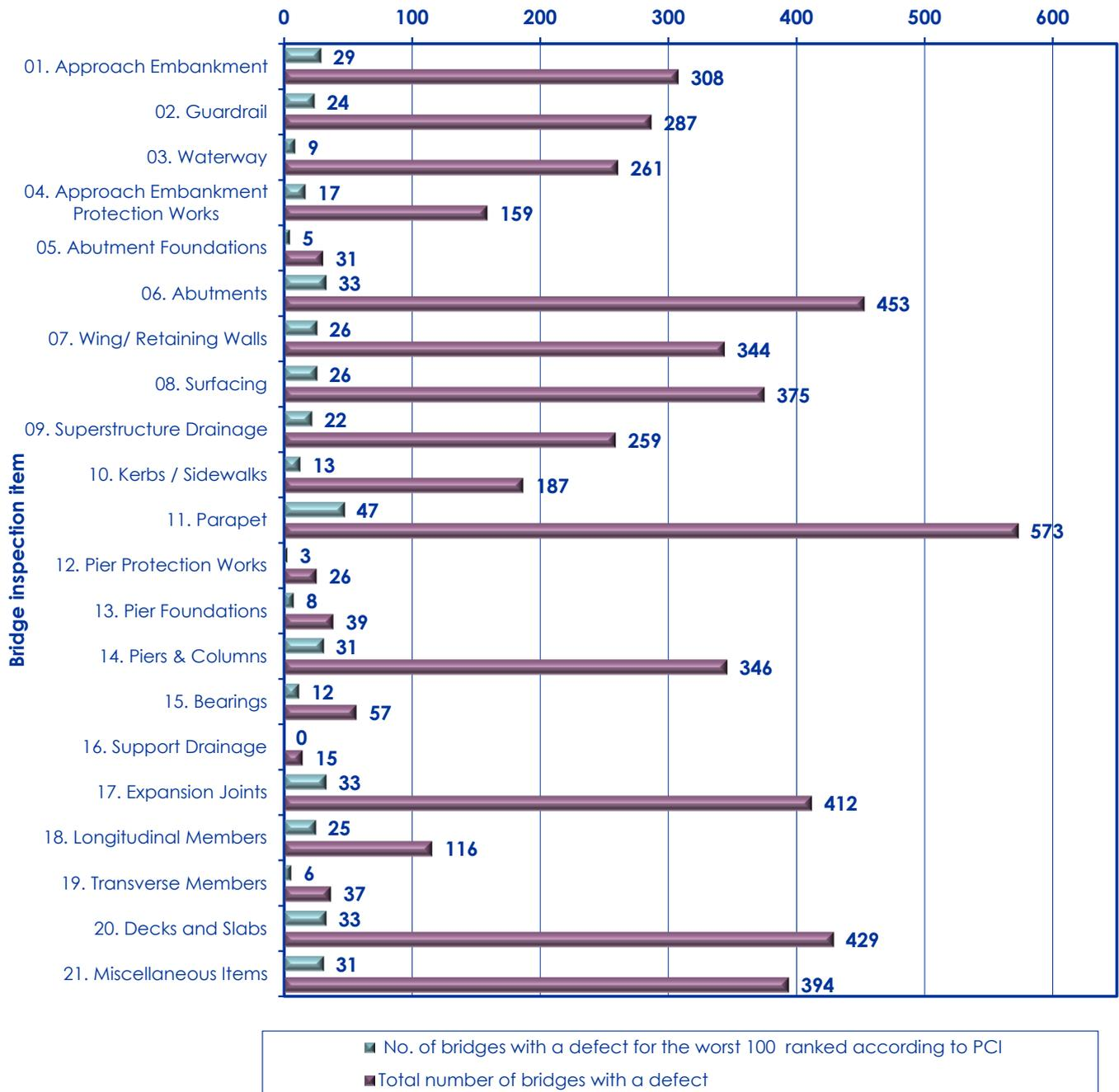
**Figure 4-13: Statistics for the defects on bridges**
