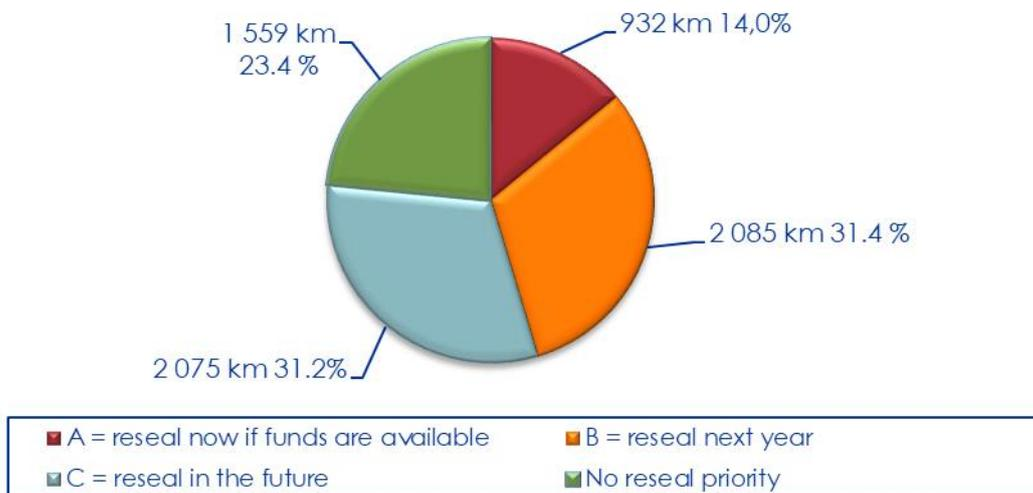
**Figure 5-9: Resealing need on paved roads according to urgency as at June 2017**
