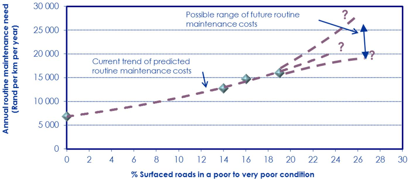
Figure 5-46: Routine maintenance cost versus condition of the paved road network
