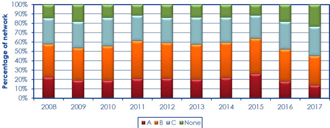
**Figure 4-30: Resealing demand of paved roads according to urgency 2007 to 2017**
