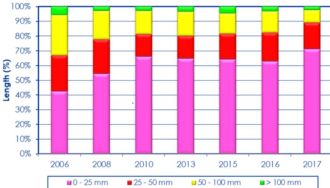
Figure 4-29: Gravel thickness distribution on unpaved roads 2006 to 2017
