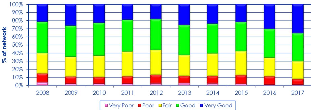
Figure 4-21: Change in the VCI by road length of the paved road network 2008 to 2017
