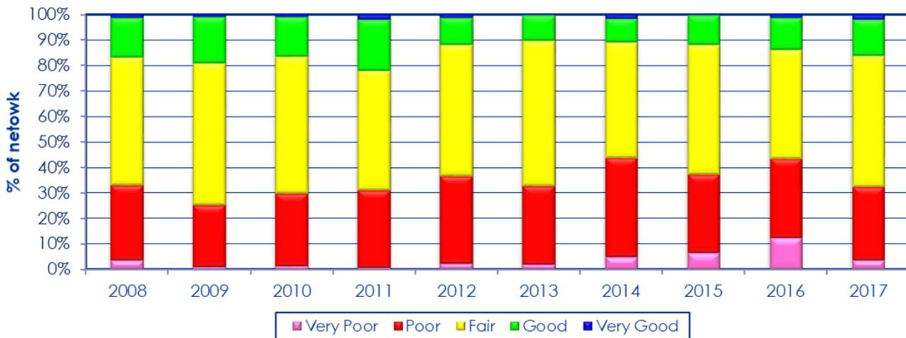
Figure 4-25: Change in the visual condition by road length of maintained unpaved road network 2008 to 2017
