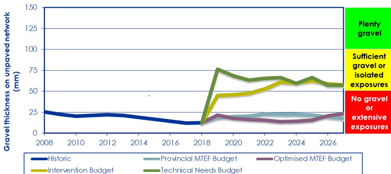
**Figure 5-35: Average gravel thickness of maintained unpaved roads**
