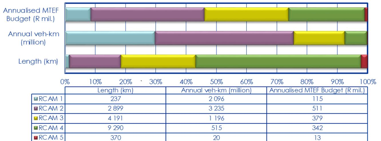
Figure 5-29: Road network according to RCAM classification versus the Optimised MTEF Budget allocation
