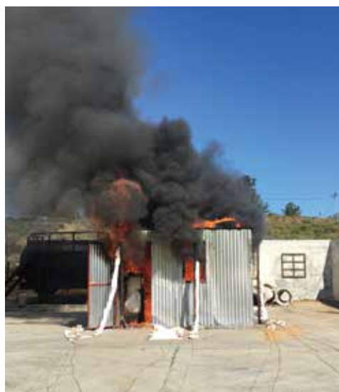
Figure 11: Instrumented shack during the “representative” full scale flaming fire tests
