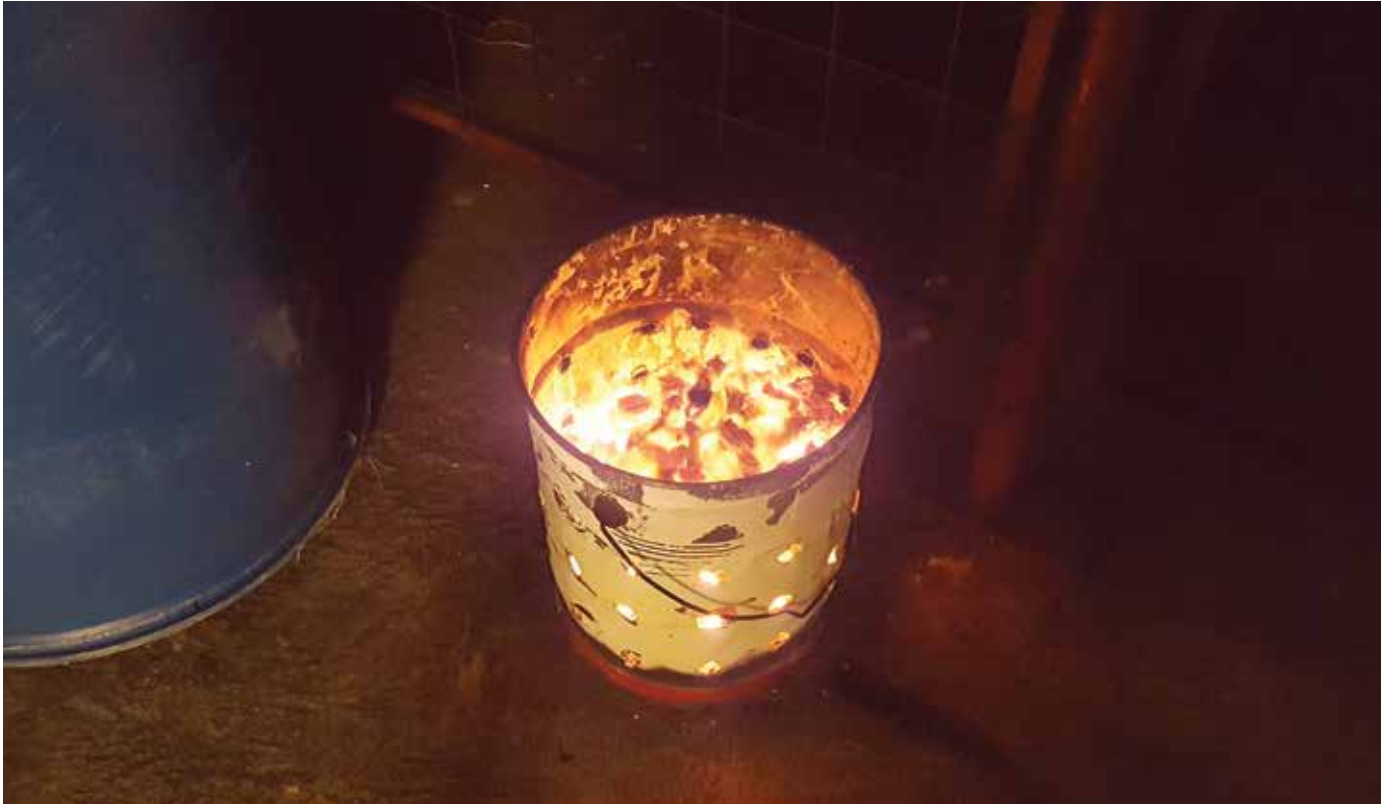
Figure 18: An example of an mbawula which was used in the nuisance testing
