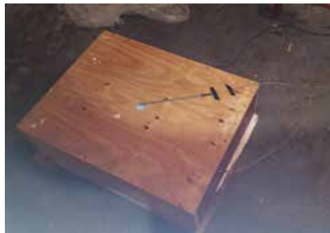
Figure 10: a) Smoke generator setup for smouldering fire test (a) Initially, and after smouldering test
