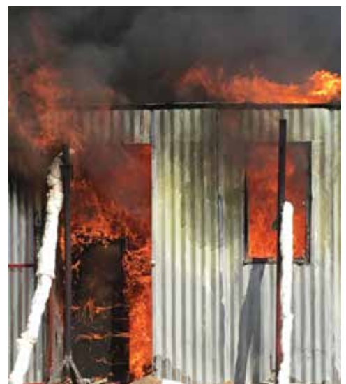
Figure 11: Instrumented shack during the “representative” full scale flaming fire tests
